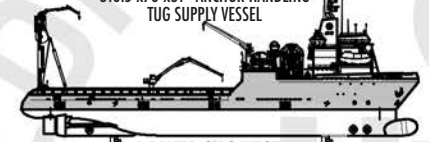
LANEY CHOUEST 348'x72'x31' ANCHOR HANDLING TUG SUPPLY VESSEL
