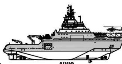
AIVIQ 360.7'x80'x34' A3 ICE ANCHOR HANDLING TUG SUPPLY VESSEL
