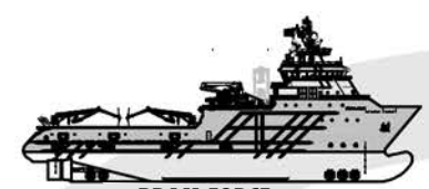
BRAM FORCE 307'x72'x31' ANCHOR HANDLING TUG SUPPLY VESSEL
