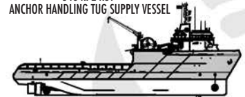
MAX CHOUEST JOSHUA CHOUEST 288'x66'x23' ANCHOR HANDLING TUG SUPPLY VESSEL
