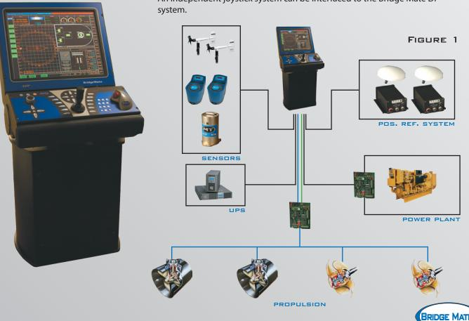
An independent joystick system can be interfaced to the Bridge Mate DP
